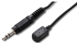
Figure 5 – IR Emitter Cable CIR-EMT (Emitter has adhesive backing) Pin out: Tip=Anode, Ring=Cathode, Sleeve=Not Connected
