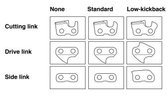
Combining these links in different ways gives different degrees of kickback reduction. In terms of kickback reduction alone, four different types of link are available.
