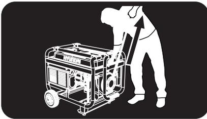
4. **ALL GENERATORS:** If starting manually, grasp the recoil starter handle and pull it until the generator starts. Do not allow the recoil starter to snap back. Return it slowly by hand.
