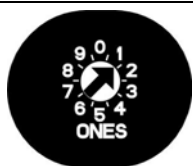
Figure 34: B810 Switch Set to Address 1
