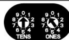
Figure 29: B208 Switches Set to Address 9
