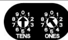
Figure 30: B308 Switches Set to Address 9
