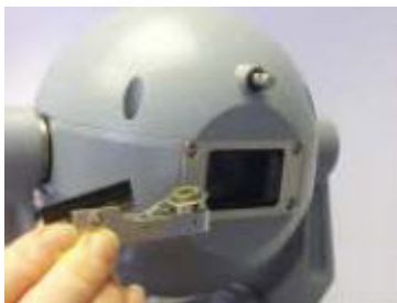
Figure 2.9: Remove wiper-arm from wiper shaft
