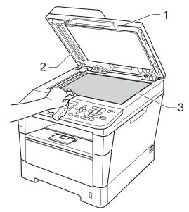
4 In the ADF unit, clean the white bar (1) and the scanner glass strip (2) underneath it with a soft lint-free cloth moistened with water.
