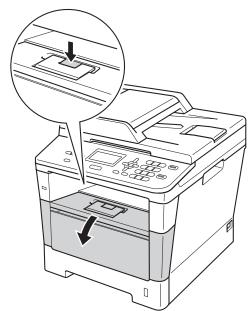
3 Slowly take out the drum unit and toner cartridge assembly. The jammed paper may be pulled out with the drum unit and toner cartridge assembly, or this may release the paper so you can pull it out from inside of the machine.
