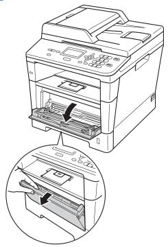
3 Pull out the MP tray support (1) and unfold the flap (2).
