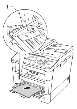
4 Lift up the support flap to prevent paper from sliding off the face-down output tray, or remove each page as soon as it comes out of the machine.
