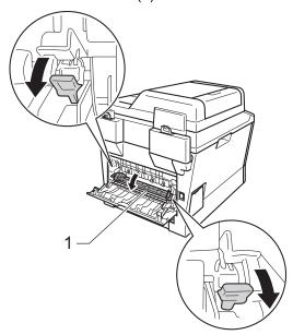
6 Using both hands, gently pull the jammed paper out of the fuser unit.
