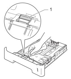
Wipe the two pick-up rollers (1) inside the machine to remove dust.
