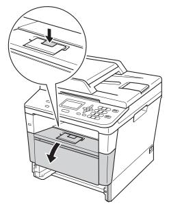
5 Slowly take out the drum unit and toner cartridge assembly. The jammed paper may be pulled out with the drum unit and toner cartridge assembly, or this may release the paper so you can pull it out from inside of the machine.
