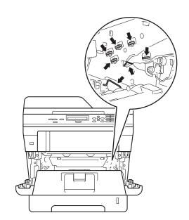
6 Push down the green lock lever and take the toner cartridge out of the drum unit. Remove the jammed paper if there is any inside the drum unit.
