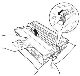
7 Turn the drum unit as shown in the illustration. Make sure that the drum unit gear (1) is on the left hand side.
