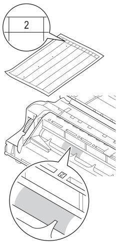
9 Turn the drum unit gear toward you by hand while checking the surface of the suspected area.
