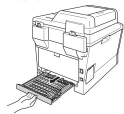
7 Pull the jammed paper out of the machine or out of the duplex tray.
