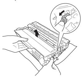
7 Put the toner cartridge back into the drum unit until you hear it lock into place. If you have put the cartridge in correctly, the green lock lever will lift automatically.
