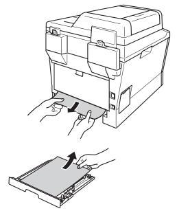
8 Make sure that the jammed paper does not remain under the machine from static electricity.
