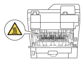
Pull the green tabs at the left and right hand sides toward you and fold down the fuser cover (1).
