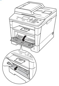
2 Pull out the MP tray support (1) and unfold the flap (2).
