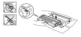
Clean the primary corona wire inside the drum unit by gently sliding the blue tab from right to left several times. Return the blue tab to the Home position (▼) before reinstalling the drum unit and toner cartridge assembly.
