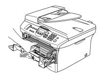
3 Hold down the lock lever on the left and pull the toner cartridge out of the drum unit.
