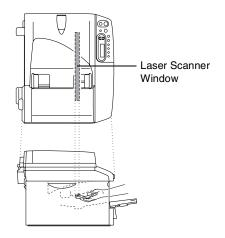
4 Put the drum unit and toner cartridge assembly back into the MFC.
