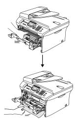
If you can not remove the drum unit and toner cartridge assembly easily, do not use extra force. Instead, lift the scanner cover, using both hands to carefully pull the jammed paper up and out of the output tray opening.
