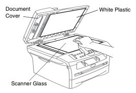
In the ADF unit, clean the white plastic bar and the scanner glass under the white bar with isopropyl alcohol on a lint-free cloth.
