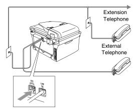
When you are using an external phone, the LCD shows Telephone.
