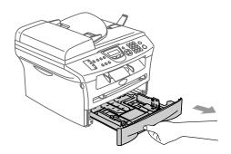
While pressing the paper guide release lever, slide the adjusters to fit the paper size.
