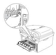
Pull the jammed paper out of the fuser unit. If the jammed paper cannot be pulled out easily, push down the tab with one hand as you gently pull out the paper with the other hand.
