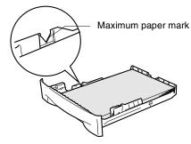
Dut the paper tray firmly back in the MFC and unfold the output paper tray support flap before you use the MFC.
