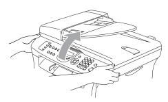
You can still use the MFC while the scanner cover is up. To close the scanner cover, push it down with both hands.
