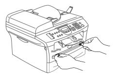
Using both hands put one sheet of paper in the manual feed slot until you feel the front edge of the paper touch the paper feed roller. Let go of the paper when you feel the MFC feed the paper in a short distance.
