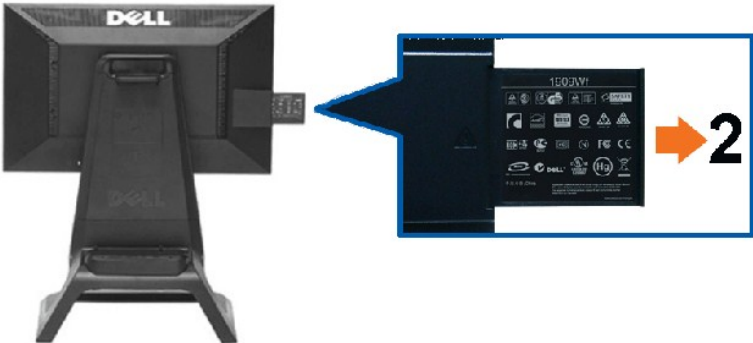
Monitor rear view with label card extended to reveal regulatory label.
