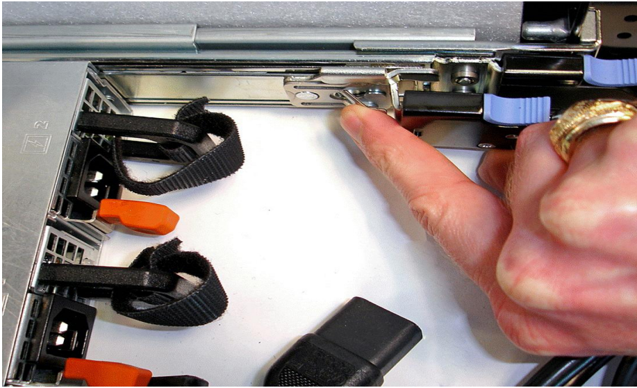
Figure 11: Replacing the Outer Power Supply
