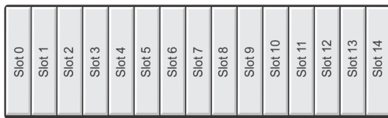
Figure 7. Dell PowerVault MD1000 Storage Enclosure Disk Slots
