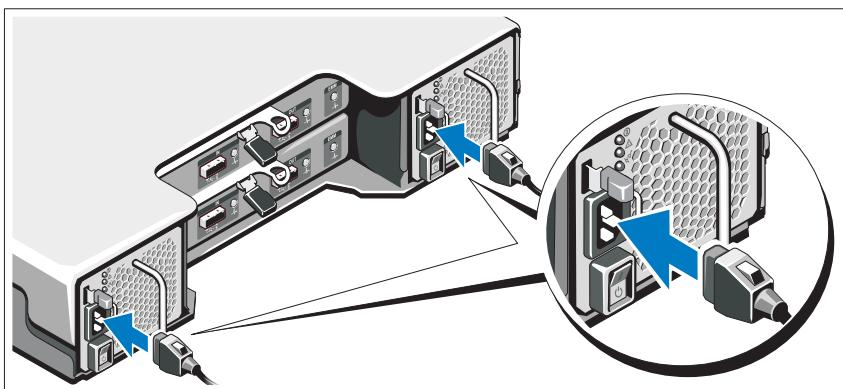
Ensure that the power switch is in the OFF position before connecting the power cable(s). Connect the system's power cable(s) to the system.
