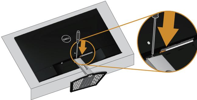
4. While pressing on the release button, pull the stand out.
