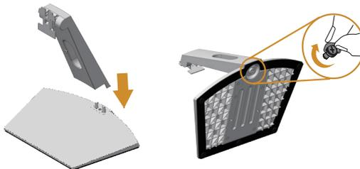
3. Fit the two tabs on the upper part of the stand to the groove on the back of the monitor. Press the stand until it snaps into place.
