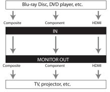
When choosing a connection format, bear in mind that the receiver does not convert between formats, so only outputs of the same format as the input will output the signal.
