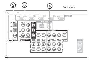
Connect your components to the appropriate jacks. The default input assignments are shown below. To change assignments, see "Setting up Component input (Component menu)" on page 22.
