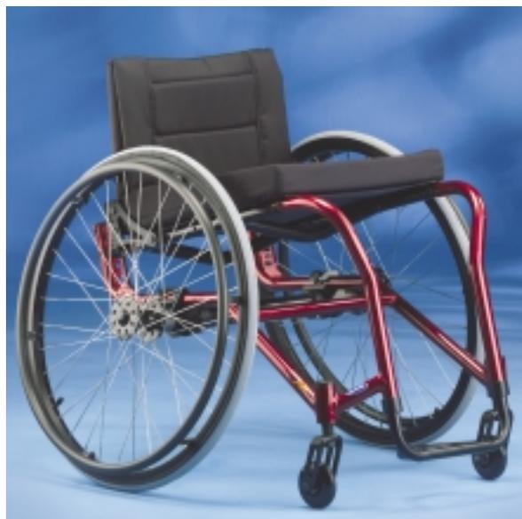
The Electric Red A4 rigid wheelchair shown has a tapered front end, 24” high performance spoked wheels with Primo™ tires, aluminum anodized handrims, one-piece adjustable angle footboard and 3” rollerblade casters.
