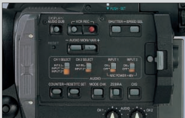
Sub-panel (with LCD monitor opened)
