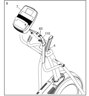
9. **Tip: Avoid pinching the wires.** Attach the Console (7) to the Upright (4) with four M4 x 16mm Screws (101).
