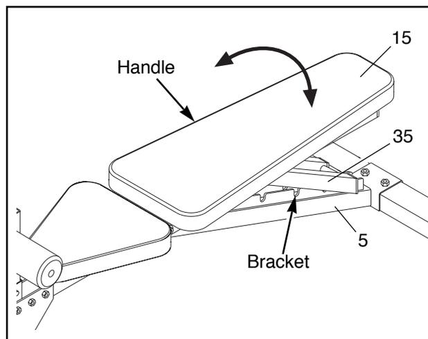
**⚠ WARNING:** Be sure the Backrest Adjustment Bracket is securely locked to the Bench Frame before using the weight bench.
