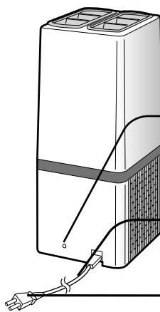
Use a pointed object, e.g a pen tip, to press this button after replacing Plasmacluster Ion Generating Unit.
