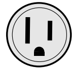
Two-Pole, 3-wire Grounding Receptacle 15 Amps. 125V.
