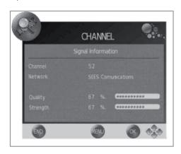
Position and align the antenna so that the maximum possible values for "Quality" and "Strength" are obtained.
