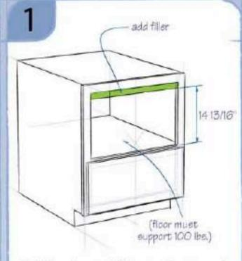
Add horizontal filler to the top of the opening. Height of opening should be 14 13/16".
