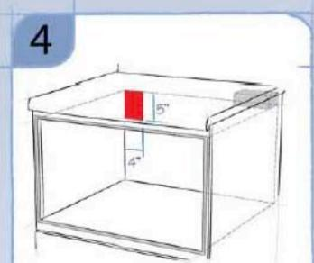
Place electrical outlet in upper back left side in the cavity opening. Can also be installed using an electrical outlet in an adjacent cabinet. Always check electrical codes for requirements.
