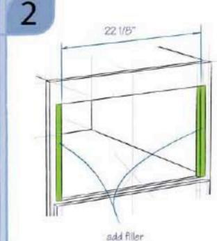
Add vertical fillers to the opening width. The width of the opening should be 22 1/8".
