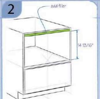
Add horizontal filler to the top of the opening. Height of opening should be 14 13/16".
