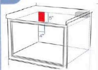
Place electrical outlet in upper back left side in the cavity opening. Can also be installed using an electrical outlet in an adjacent cabinet. Always check electrical codes for requirements.
