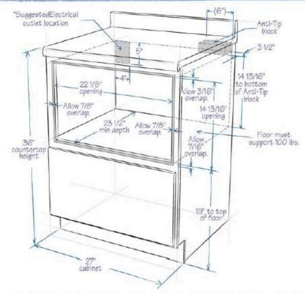
\* Can also be installed using an electrical outlet in an adjacent cabinet within the area where the provided electrical cord can reach. Fower cord access hole in cabinet should be a minimum 1 1/2" diameter hole and deburred of all sharp edges.
