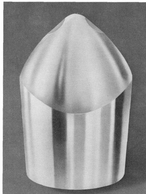
WORN HYPERELLIPTICAL STYLUS FIGURE 4B
