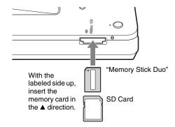
Push the memory card into the slot until you hear a click. To remove, push the card and pull out.
