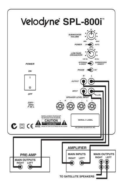
Figure 2. Installation Using Stereo Line-Level Inputs
