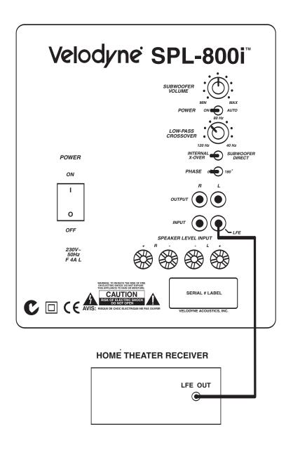
Figure 1. Installation Using LFE Line-Level Inputs
