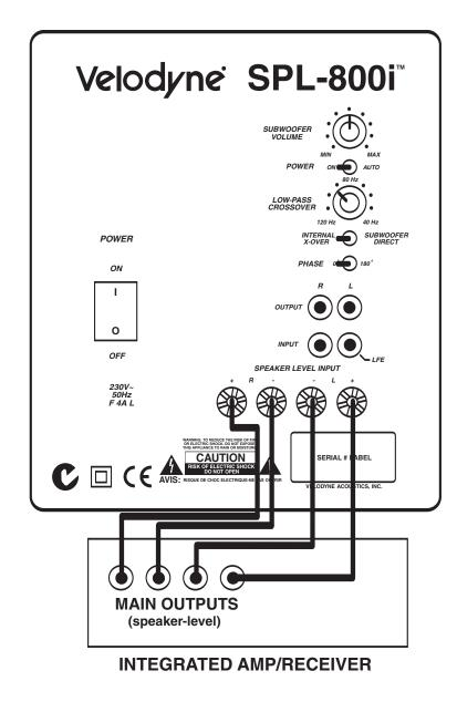
Figure 3. Installation Using Speaker-Level Inputs
