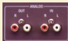
Analog Input/Output Terminals
