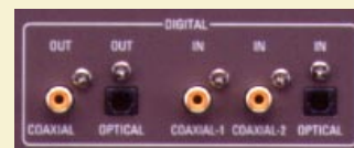
Digital Input/Output Terminals
