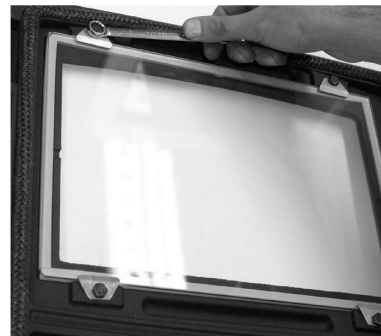
Fig. 19. Tightening the glass clips
