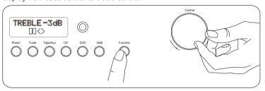
**Attention:** Please note that due to the level of boost available on this treble control, please be aware that prolonged use of this amplifier at high levels with an increased treble content may cause permanent damage to your speakers. Please operate this system within the safe working limits of any ancillary equipment that is connected to it.
