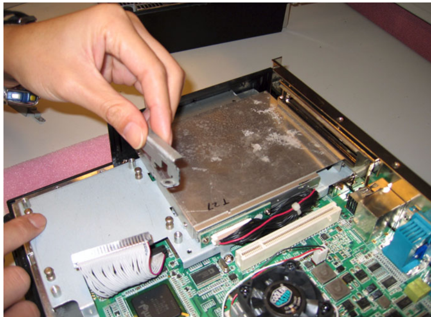
Figure A.14 Removing the fixed brace
