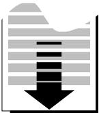
PGE END lets you tell the printer whether or not to use the LENG (form length) setting to determine the last printing line on a cut sheet. You can select *Off* to let printing continue beyond the LENG setting; or *On* to specify that printing stop at the LENG setting. A third setting is *Roll*, which you can select to feed unsprocketed roll paper into the printer. When you select *Roll*, printing is continuous without regard for page length.
