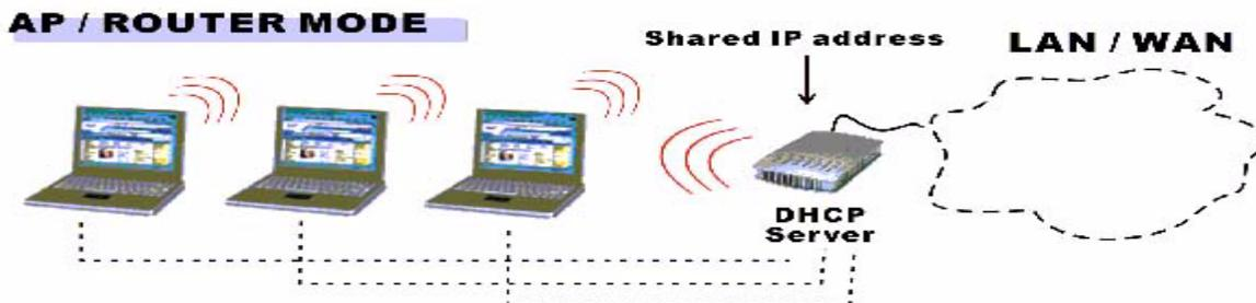
**Figure 3. AP/Router Mode Configuration**
