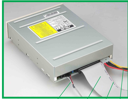
CD/DVD-ROM Audio Cable IDE Ribbon Cable Red Stripe to Pin 1 Power Cable (P4)
