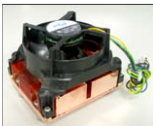
CPU heatsink (top view)
