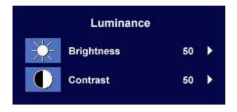
Press ◀ or ▶ key to adjust the degree of Brightness, press "Exit" to return to the previous menu.
