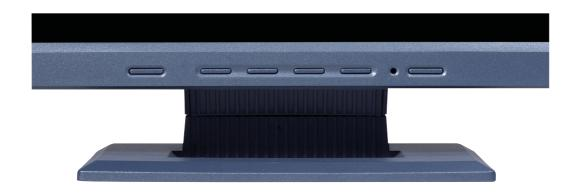
There are 6 keys for user's control including "*iKey*", "Exit", "Enter", "<" and ">" key and a power swith. The following descriptions are the introduction of these keys & switch.
