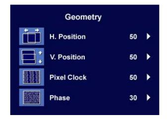
Press ◀ or ▶ key to adjust the Horizontal Position, press "Exit" to return to previous menu.
