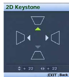
The values on the lower portion of the page change while pressing. When the values reach their maximum or minimum with repeated button presses, the image's shape will stop changing. You will not be able to change the image further in that direction.
