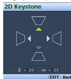
6. Based on the image shape displayed on the screen, press the keystone buttons (**◻ / ▲ Up**, **◻ / ◀ Left**, **◻ / ▼ Down**, **◻ / ▶ Right**) to adjust the image to a rectangular or square one.
