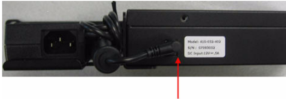
Figure 15 Insert the power supply cable into the connector on the rear panel
