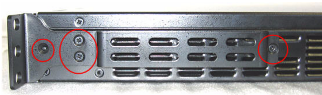
Figure 28 Each bracket is attached to the side of the ET1000A using four screws
