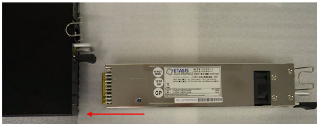
Figure 37 Slide the replacement power supply into the slot on the rear panel
