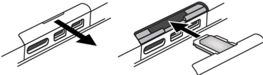
1. Remove the micro SIM card tray from the back of your tablet.
