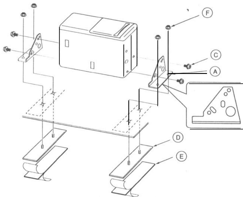
Hängender Einbau . Suspended Installation . Installation suspendue . Montaggio sospeso .
