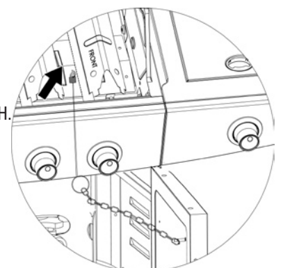
Main Burner Lighting Rod Placement
