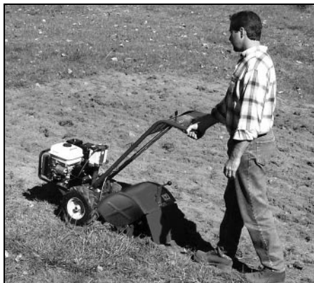
Figure 4-2: Guiding the tiller with one hand.
