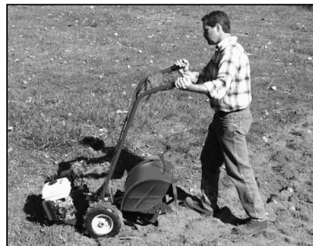
Figure 4-3: Find balance point before turning.
