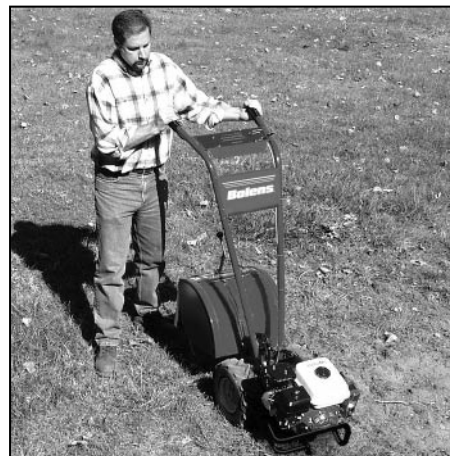
Figure 4-4: Push handlebars sideways to turn tiller.
