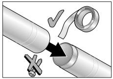
All joints should be tight to avoid leaks. The male end of each duct section must point away from the dryer.
