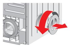
2. Remove the bayonet ring from the rear panel and attach it to the side panel vent.
