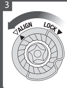
3 Unlock Top Burr. Grip the handle and turn anti-clockwise
