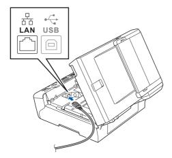
Carefully route the network cable through the trench and out the back of the machine. Then, connect the cable to your network.
