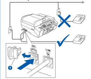
Set the receive mode to External TAD if you have an external answering machine. See Choose the correct Receive Mode on page 8. For additional details, see Connecting an external TAD (telephone answering device) in Chapter 7 of the User's Guide.
