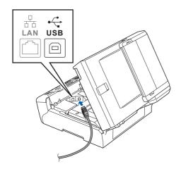
Carefully route the USB cable through the trench and out the back of the machine as shown below and connect the cable to your computer.
