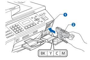
Install each ink cartridge in the direction of the arrow on the label.
