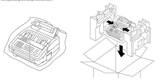
7. Place any documents (manual and printed materials) and the drum unit and toner cartridge assembly into the carton box as shown below. If you are shipping the MFC, insert your documentation explaining the reason.
