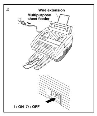
1) Turn off the power switch and unplug the power cord.
