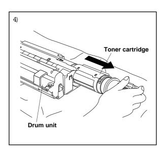
4) Remove the toner cartridge from the drumunit and keep it in a safe place. For more information, see "Replacing the Toner Cartridge" on page 12-1~4.
