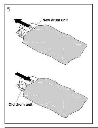
5) Wait to unpack the new drum unit until immediately before installing it. Place the old drum unit into the aluminum bag and discard it according to local regulations.
