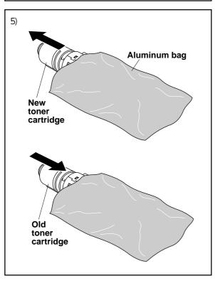
5) Unpack the new toner cartridge. Place the used toner cartridge into the aluminum bag and discard it according to local regulations.
