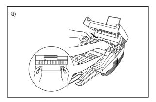
8) Holding the new drum unit by its handles, install it. Close the top cover.
