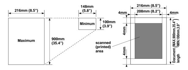
The size of the documents you want to send by fax should not be larger (or smaller) than your MFC can accommodate. The documents should each be between 5.8 and 8.5 inches (148 and 216 mm) wide and between 3.9 and 35.4 inches (100 and 900 mm) larg.
