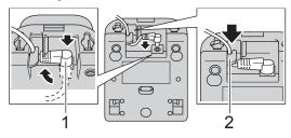
Plug the AC adapter into the electrical socket.
