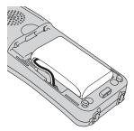
5 Install the battery cover by sliding it onto the back of the handset.
