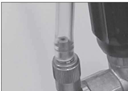
Figure 2 - Attach suction tube to barb fitting
