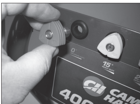
Figure 3 - Insert spray tips into the holder
