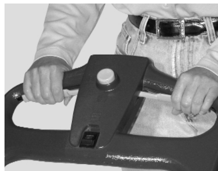
Figure 18. Step 3: Release the start button
