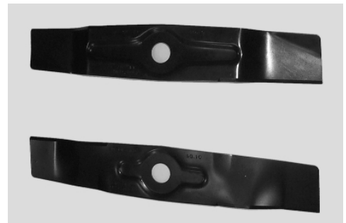
Figure 30. Comparing the cutting blade (top) with the mulching blade (bottom)
