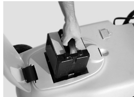
Figure 21. Inserting the battery
