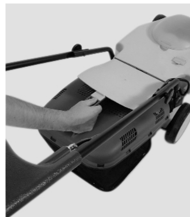
Figure 28. Attaching the rear bagger
