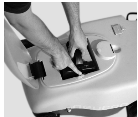
Figure 20. Removing the battery
