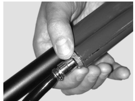
Figure 8. Hand-tightening the locking nut
