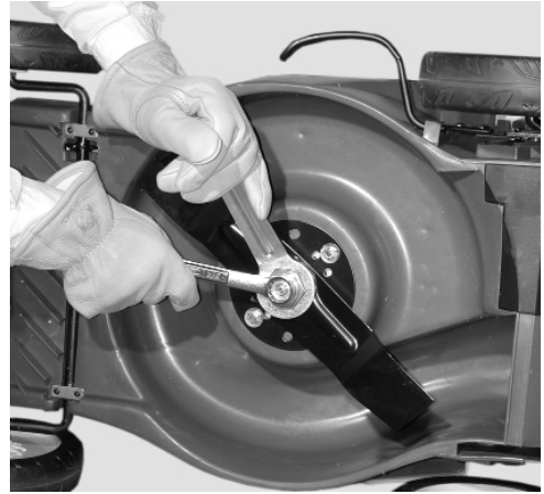
Figure 31. Removing the blade
