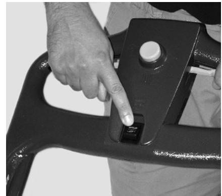
Figure 14. Pushing the Mower/Auxiliary switch to the Mower setting
