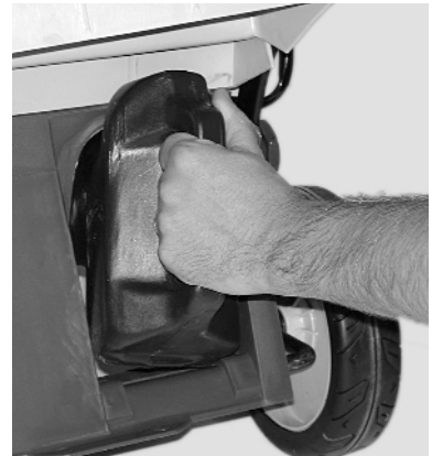
Figure 29. Installing the mulching plug
