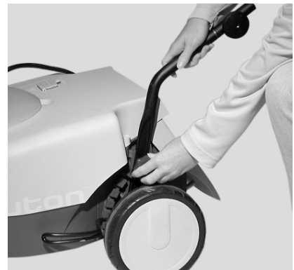
Figure 2. Attaching the lower left handlebar
