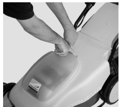
Figure 5. Opening the battery cover
