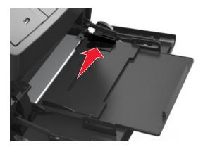
**Note:** Use the paper size indicators on the bottom of the tray to help position the guides.
