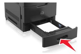
**8** From the printer control panel, set the paper size and type in the Paper menu to match the paper loaded in the tray.
