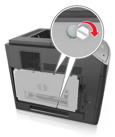
**7** Reattach the controller board access cover.
