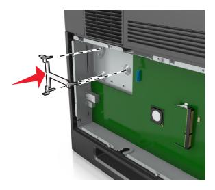
**Note:** Make sure that the plastic bracket has latched completely, and that the plastic bracket is seated firmly on the controller board cage.
