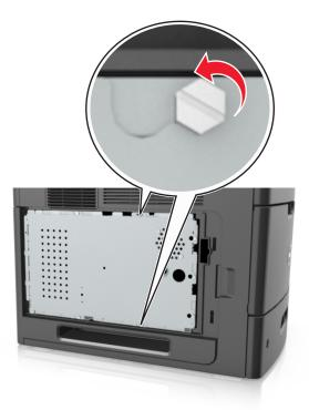
**3** Remove the controller board shield.
