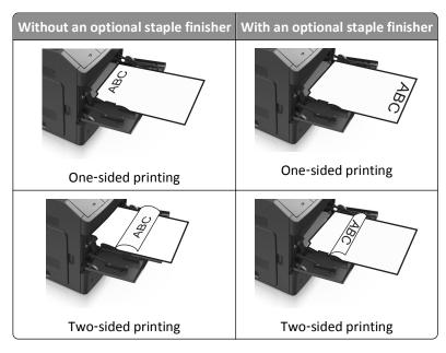
• Load envelopes with the flap side down and on the left of the multipurpose feeder.
