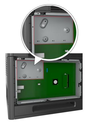
Note: If an optional ISP is currently installed, then the printer hard disk must be installed onto the ISP.
