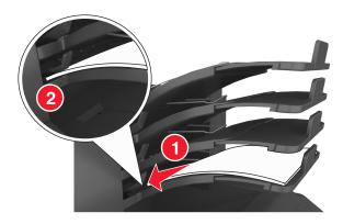
Note: If the paper is not under the bin arm, then a jam occurs due to an overfilled bin.
