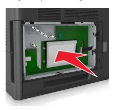
**b** Use the two provided screws to attach the printer hard disk mounting bracket.
