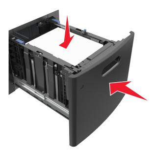
**6** From the printer control panel, set the size and type in the Paper menu to match the paper loaded in the tray. **Note:** Set the correct paper size and type to avoid paper jams and print quality problems.
