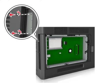
4 Remove the printer hard disk.
