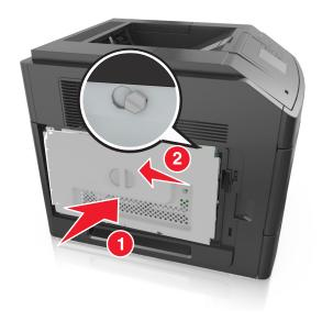
**6** Tighten the screws on the controller board shield.
