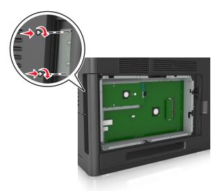
**c** Insert the plug of the printer hard disk interface cable into the receptacle of the controller board.
