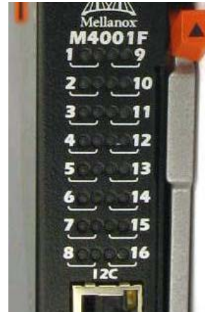
Figure 2: Physical and Logical Link Indication LEDs
