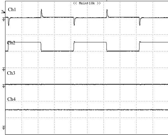
Figure 9: Output voltage response to step-change in load current Iout2 (75%-50%-75% of Io, max; di/dt = 2.5A/μs) at Iout1=7.5A. Load cap: 470μF, 35mΩ ESR solid electrolytic capacitor and 1μF ceramic capacitor. Ch1=Vout2 (100mV/div), Ch2=Iout2 (7.5A/div), Ch3=Vout1 (100mV/div), Ch4=Iout1 (7.5A/div) Scope measurement should be made using a BNC cable (length shorter than 20 inches). Position the load between 51 mm to 76 mm (2 inches to 3 inches) from the module.
