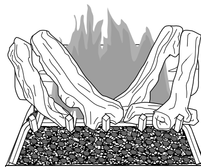
Figure 42 - Typical Flame Pattern
